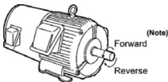
(Note) The rotational direction of IEC-compliant motors is opposite to that of the motor shown here.
