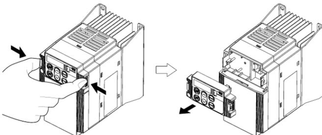
Figure 2.25 Removing a Keypad
