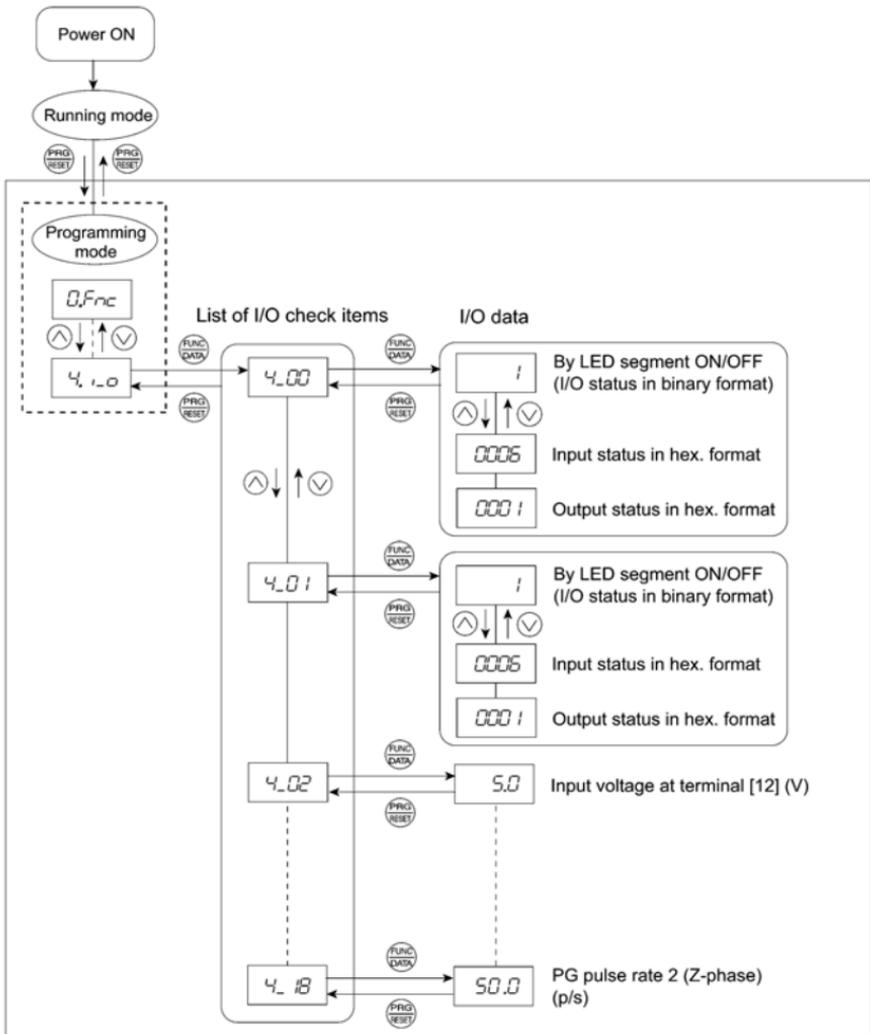
Figure 3.5 Menu Transition in Menu #4 "I/O Checking"
