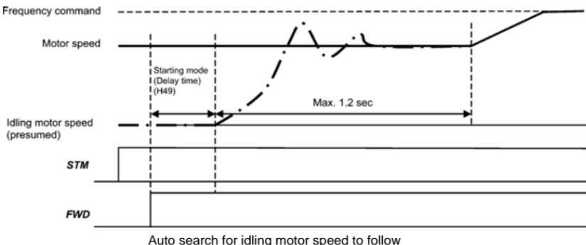
■ H09 and **STM** terminal command ("Enable auto search for idling motor speed at starting")
