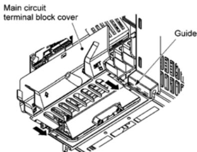
Figure 2.6 Mounting the main circuit terminal block cover
