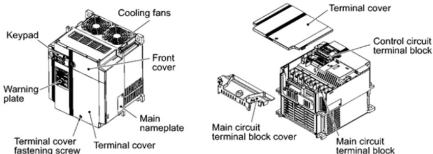
Figure 1.2 Outside and Inside Views of Inverters (FRN15E1S-2□)
