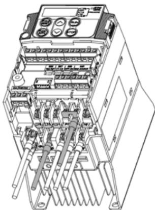
Figure 2.10 Braking Resistor Connection without DC Reactor (DCR)
