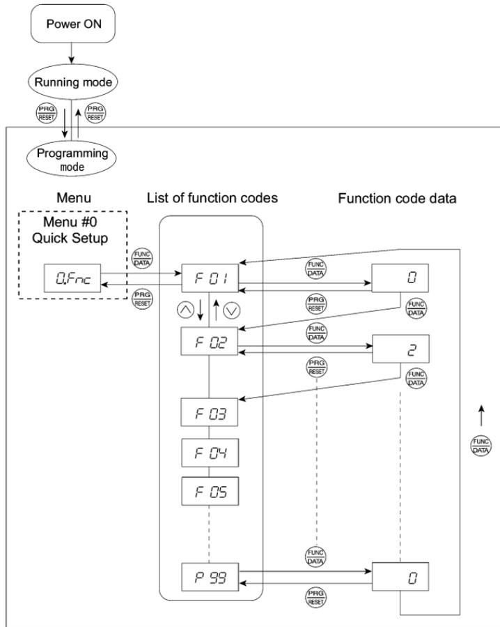
Figure 3.2 Menu Transition in Menu #0 "Quick Setup"
