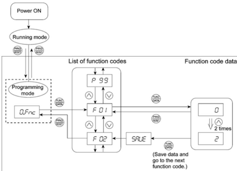
Figure 3.3 Example of Function Code Data Changing Procedure
