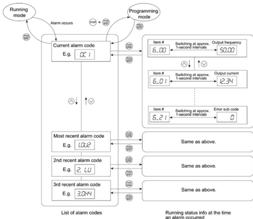
Figure 3.7 Menu Transition in Alarm Mode
