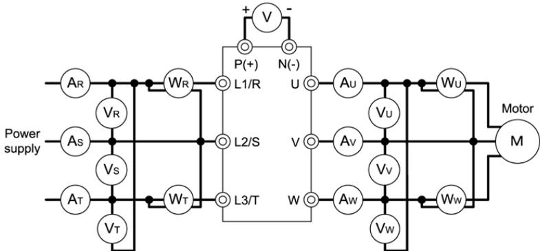
Figure 7.1 Connection of Meters
