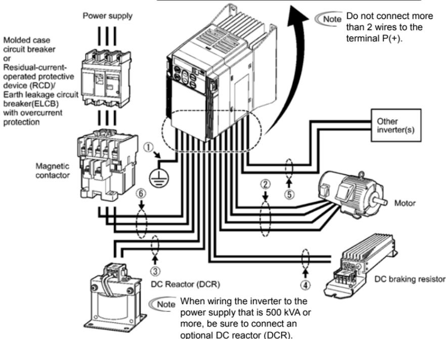
Figure 2.9 Wiring Procedure for Peripheral Equipment
