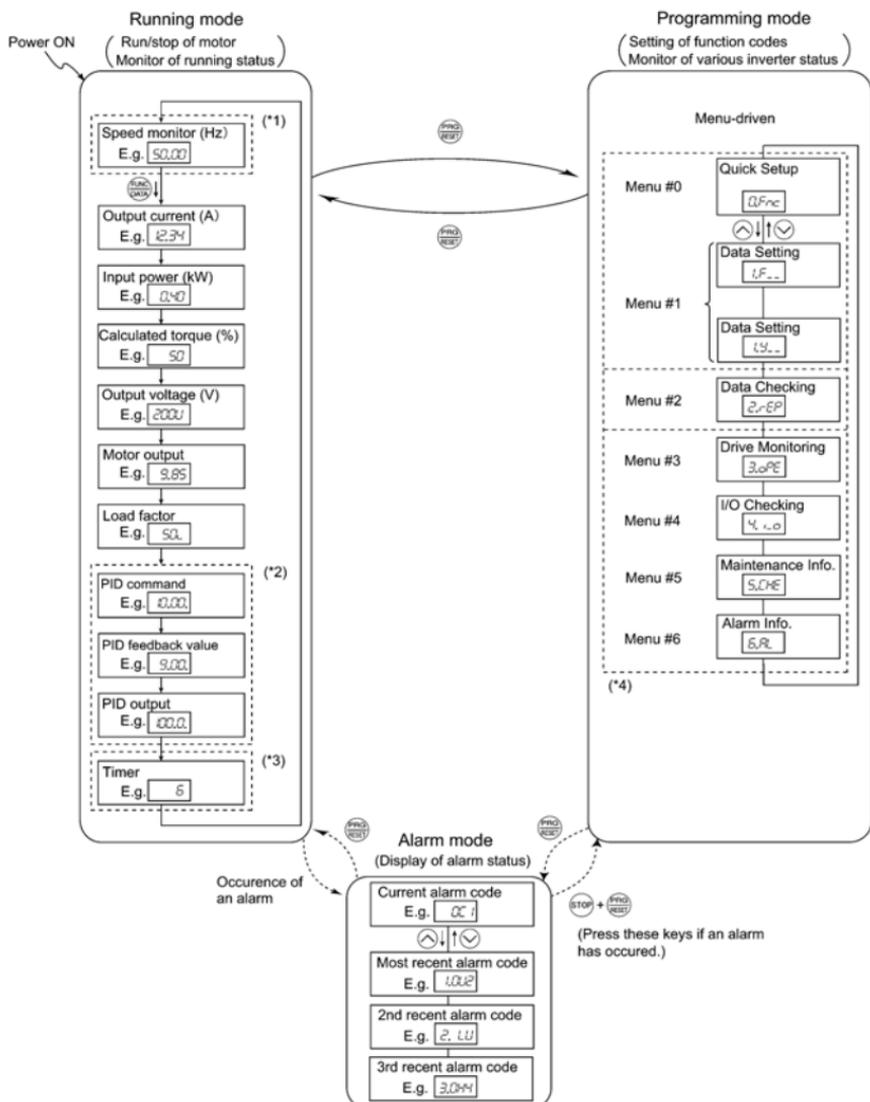
(\*1) The speed monitor allows you to select the desired one from the seven speed monitor items by using function code E48.
