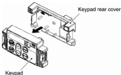
Figure 2.26 Fixing the Keypad Rear Cover for Remote Keypad Operation
