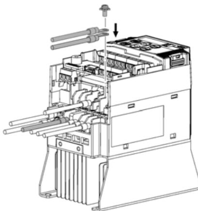
Figure 2.11 Braking Resistor Connection with DC Reactor (DCR)
