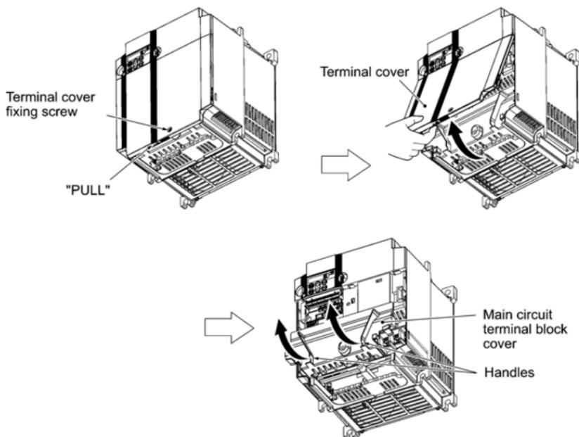
Figure 2.7 Removing the Covers (For Inverters with a Capacity of 11 and 15 kW)
