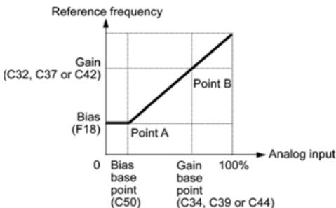
Example: Setting the bias, gain and their base points when the reference frequency 0 to 100% follows the analog input of 1 to 5 VDC to terminal [12] (in frequency command 1).
