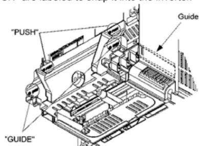
Figure 2.8 Mounting the Main Circuit Terminal Block Cover
